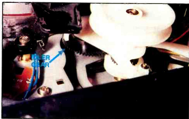
Figure 1. The notch in the VCR chassis may not be in all models to allow for easy removal of the idler gear assembly.
